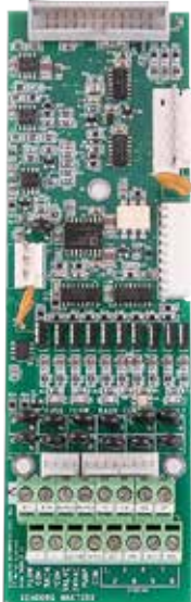
8 Station Wiring Board
